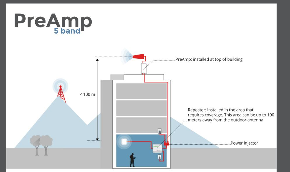
The pre-amp is installed close to the outdoor antenna to give your mobile signal that extra boost for long cable runs. You can attach a cable 100 meters long after the preamp! You can then connect directly to a machine (M2M) OR install a repeater. A repeater will give you ~5 room coverage.
