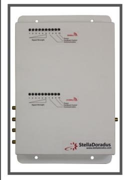
The Stella Doradus Line Amplifier is a 4 port active splitter, with a 20dB gain for use with a mobile phone repeater.
