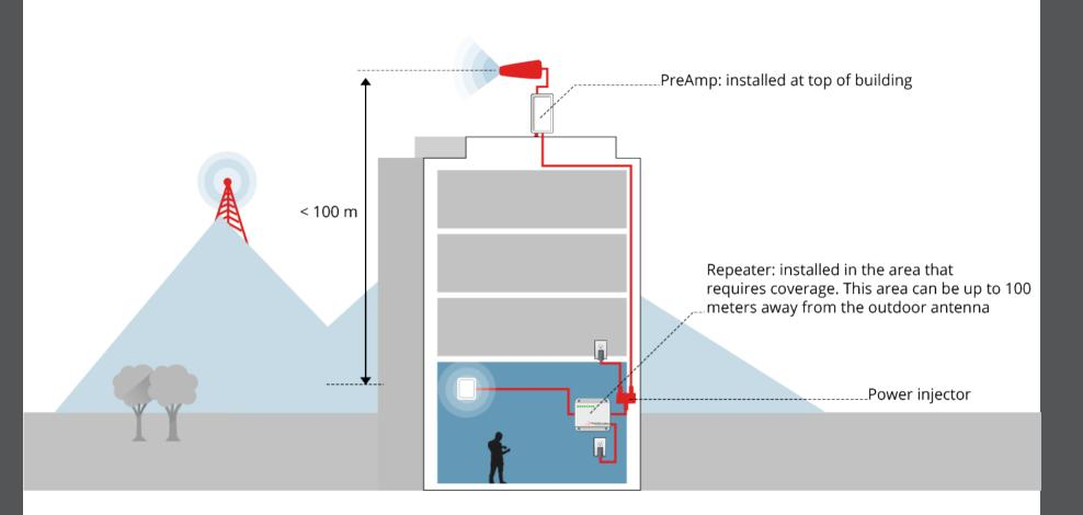
The pre-amp is installed close to the outdoor antenna to give your mobile signal that extra boost for long cable runs. You can attach a cable 100 meters long after the preamp! You can then connect directly to a machine (M2M) OR install a repeater. A repeater will give you ~5 room coverage.
