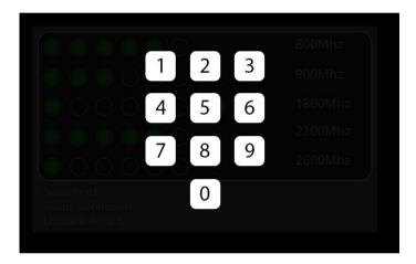
Set up pins: Admin, installer, user pin code Different levels of access Default access pin is: 8888
