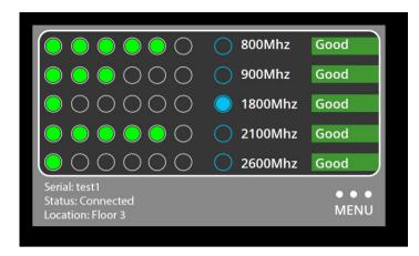
Main page: Green signal LEDs = downlink signal strength . Blue LED = Uplink switch on
